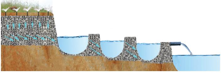
As a result of the introduction of these filter beds, 60 percent of the remaining suspended solids and 80 percent of the remaining zinc is removed from the water being discharged.
